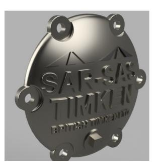
Trailing truck axle box covers above for the 7 1/4 inch 19D designed on F360 and lost wax casting in brass for the CG1, 1:24 scale 15F builds by Carel Janse van Rensburg.
