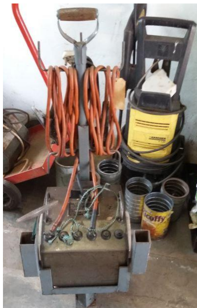
Welder with trolley and accessories
