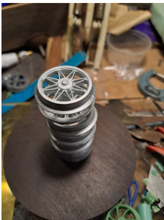
Garden railway wheels cast in zinc with the 'lost wax' casting technique by Carel Janse van Rensburg.
