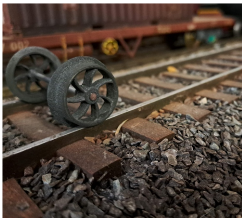
Garden railway wheels cast in zinc with the 'lost wax' casting technique by Carel Janse van Rensburg.
