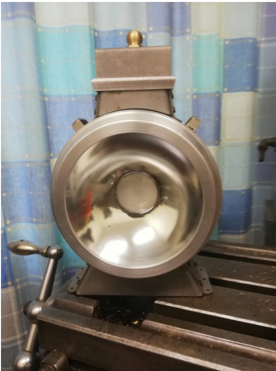
Johnny Sharpe's clinical work on detail for his Shay; the head lamp and hydrostatic lubricator.
