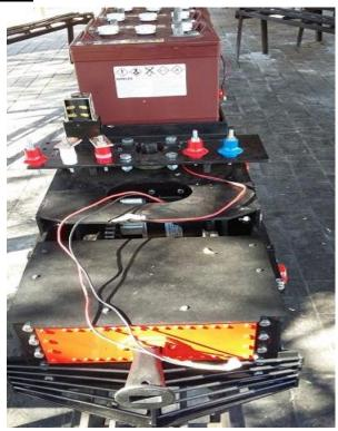
The battery frames built by the Monday gang was fitted to the locos after the few outstanding items on the bogies like chains were fitted.
