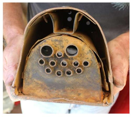
Will it pass inspection? Attached a photo of a boiler from a locomotive that had run on a private track for several years. His friend did not like the look of the boiler, so he removed it and cut it in half This is what he found.
