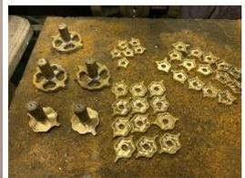
A few pictures of built up fittings made for the SAR 5 Class. Picture 0188 is of the building up of sight glasses before silver soldering, complete with stubs for machining, and image 0190 of the final machined bodies, before completing and fitting final parts like plugs. Image 0194 also show some valve bodies with machining stubs.
