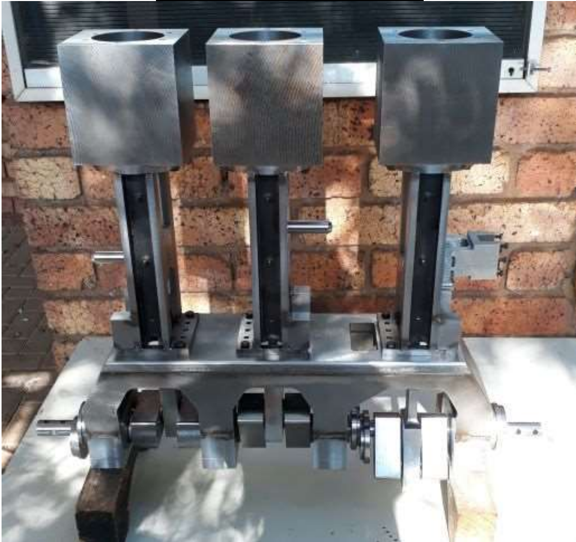
Johnny Sharpe's progress on the cylinders for his 7¼" Shay
