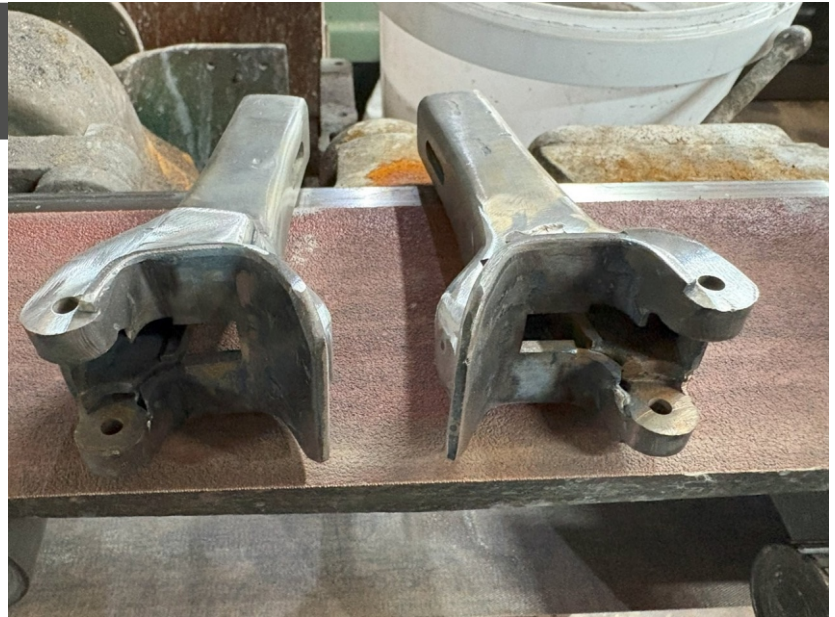
Leon's 7 1/4 inch fabricated SAR knuckle couplers
