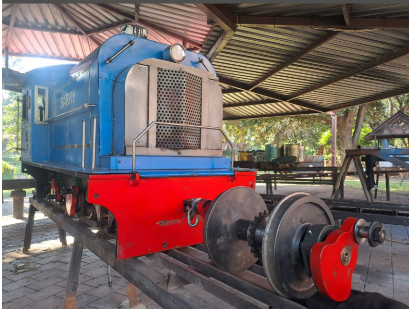
BARRY's front axle sprocket repairs
