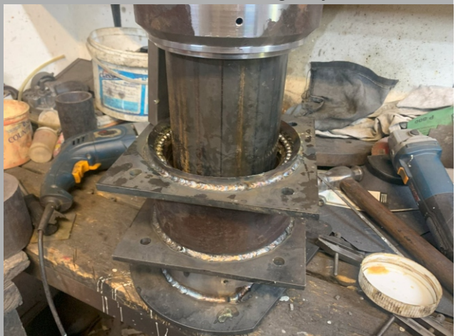
2 of the pivots for the raised track traverser at the steaming bay
