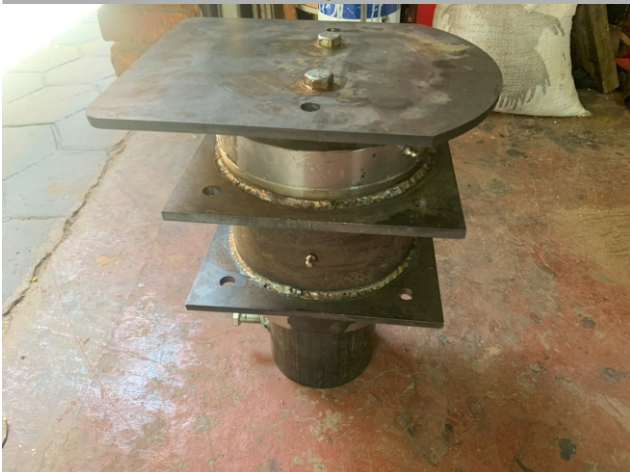
2 of the pivots for the raised track traverser at the steaming bay
