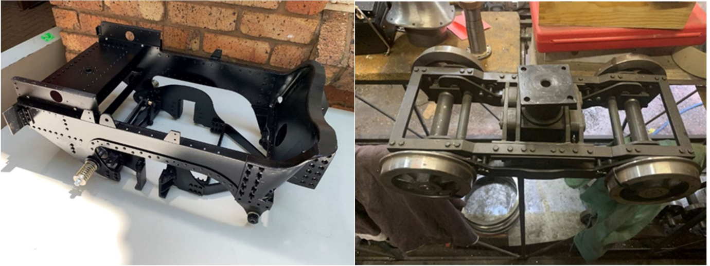
The front bogie is a typical swing link bogie used by the SAR.
