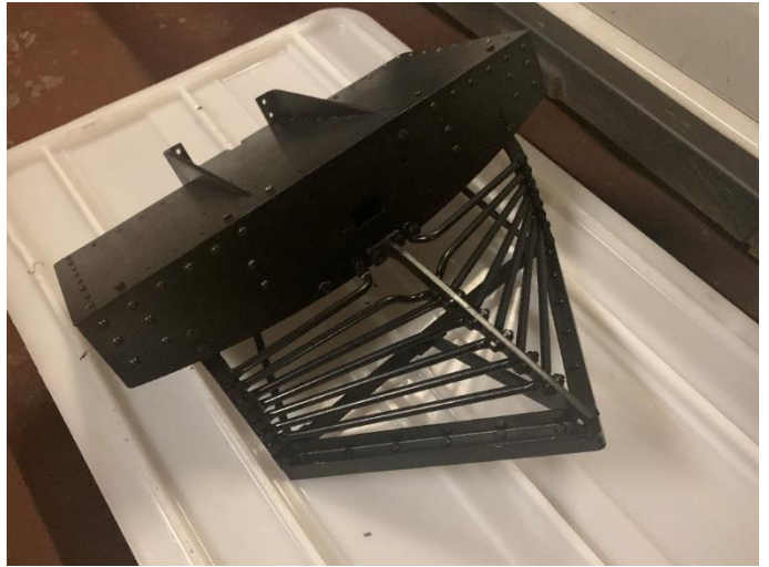
The front bogie is a typical swing link bogie used by the SAR. The distinct long cowcatcher.
