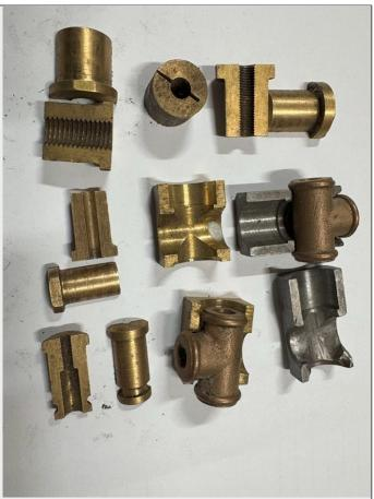
Grabbing them in the 4 jaw self centering chuck( a very good investment in saving time gripping square items), machining them round and part them off. Leaving a shoulder is important as it helps locating it in the chuck for making repeat parts. Insert the 2 pieces into the chuck and drill and tap to desired thread size.
