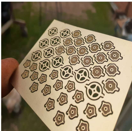
Valve handles for 15F locomotives in Cape Gauge 1, 1:24 scale.
