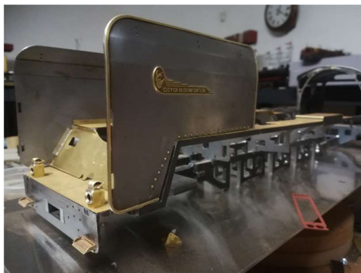
Front steps, oil lamps, smoke deflector beading and smoke deflector etched parts
