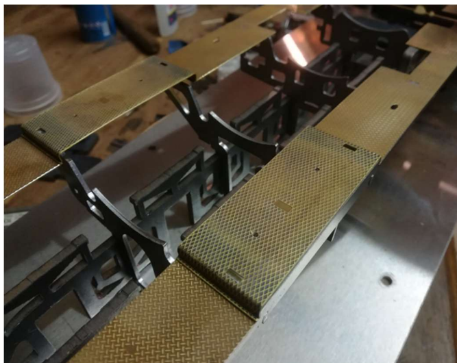
Checker and diamond plate running boards for the 15Fs in CG1, 1:24 scale.
