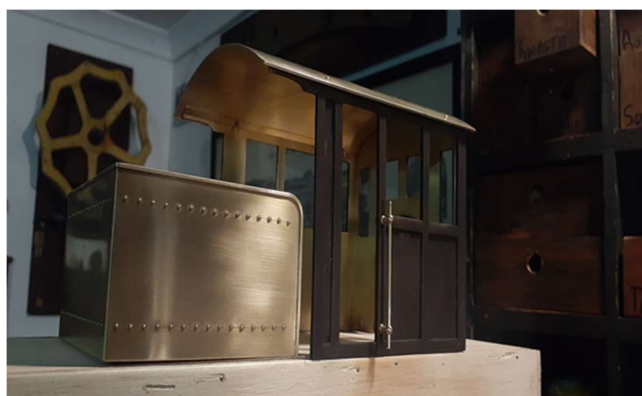
Cab and coal bunker for a live steam locomotive in 1:19 scale.
