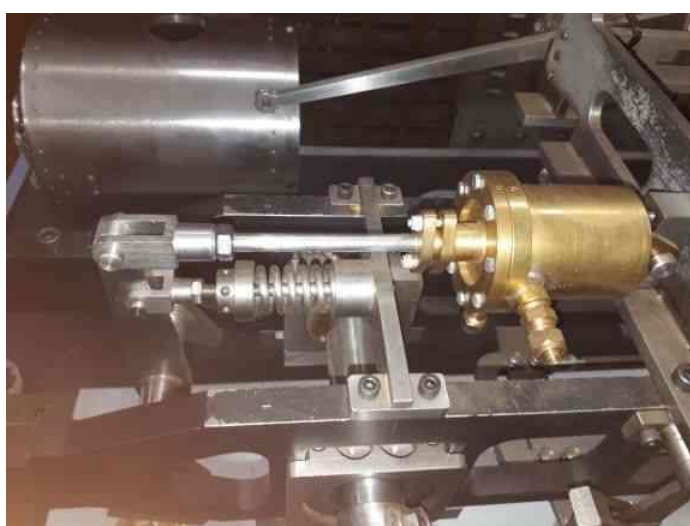
Popich switcher brake cylinder & mechanism
